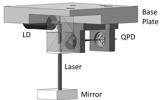
Figure 4. The physical design of autocollimator.
