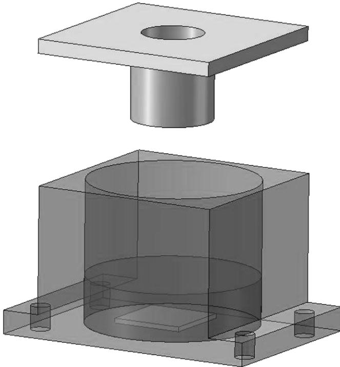
Figure 6. The leakage prevention design of top cover.
