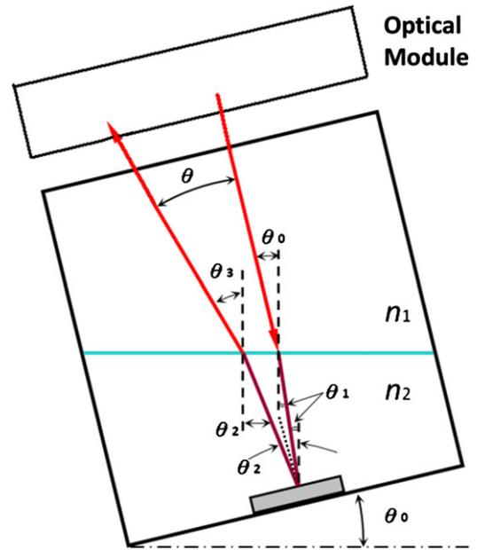
**Figure 2.** Optical path of the laser beam due to light refraction.
