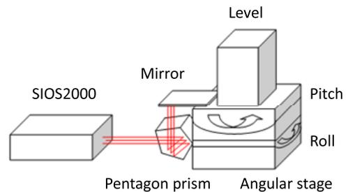
Figure 9. Setup for calibration.
