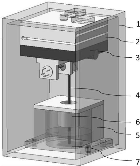
**Figure 1.** Assembled structure of dual-axis level containing: (1) frame, (2) adjustable mechanism, (3) optical module, (4) laser beam, (5) container, (6) leakage prevention tube and (7) plane mirror.
