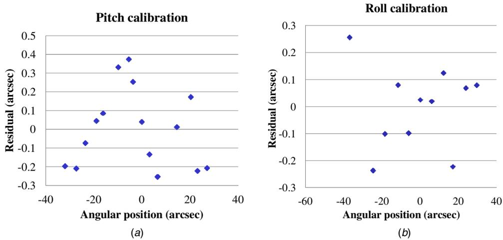
Figure 10. Residuals of  $\pm 30$  arcsec range calibration: (a) pitch and (b) roll.
