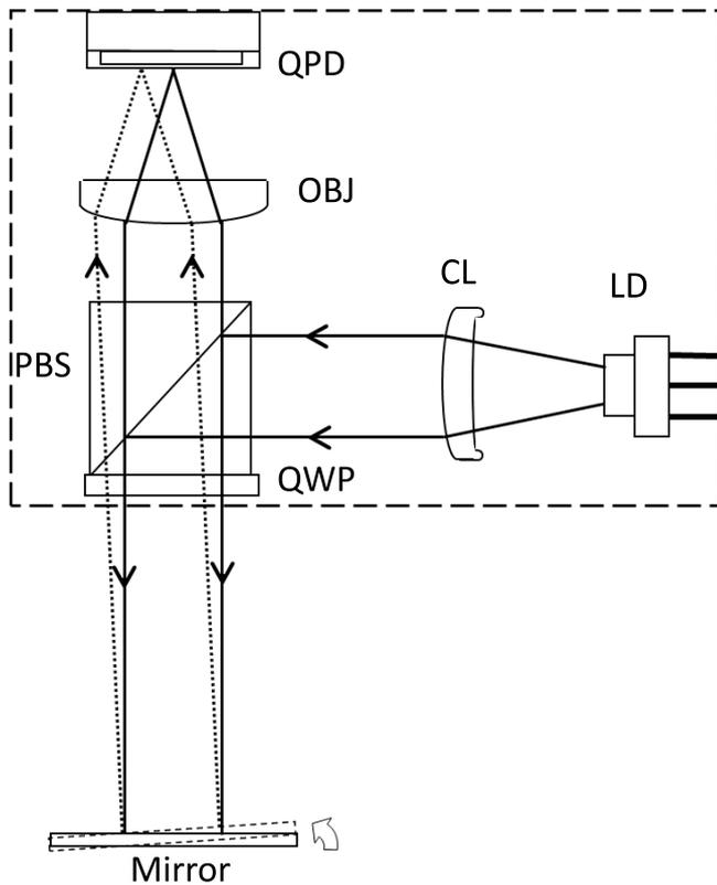
Figure 3. The principle of autocollimator design.
